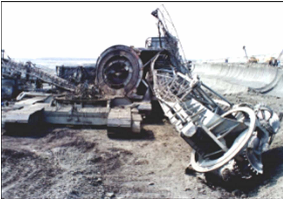
Figure 7. SRs 1200 after catastrophic failure
