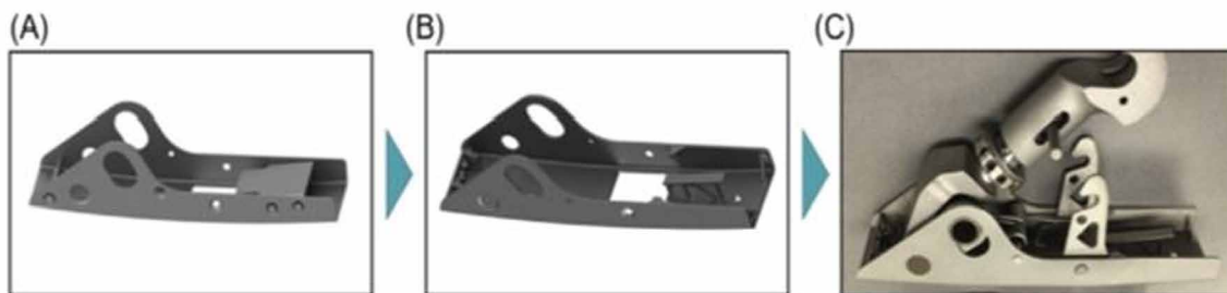
Figure 8. AM component consolidation of a jet engine cowl latch (A) initial latch handle assembly made up of 5 components, (B) AM redesigned handle with components consolidated into a single component, (C) additive manufactured jet engine cowl latch (Kamal & Rizza, 2019).
